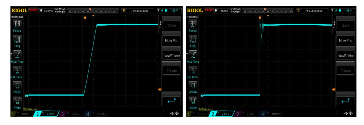
The eFuse (left) has a controlled and adjustable slew rate, reducing inrush current. The relay (right) produces noise and chatters, resulting in power loss.
