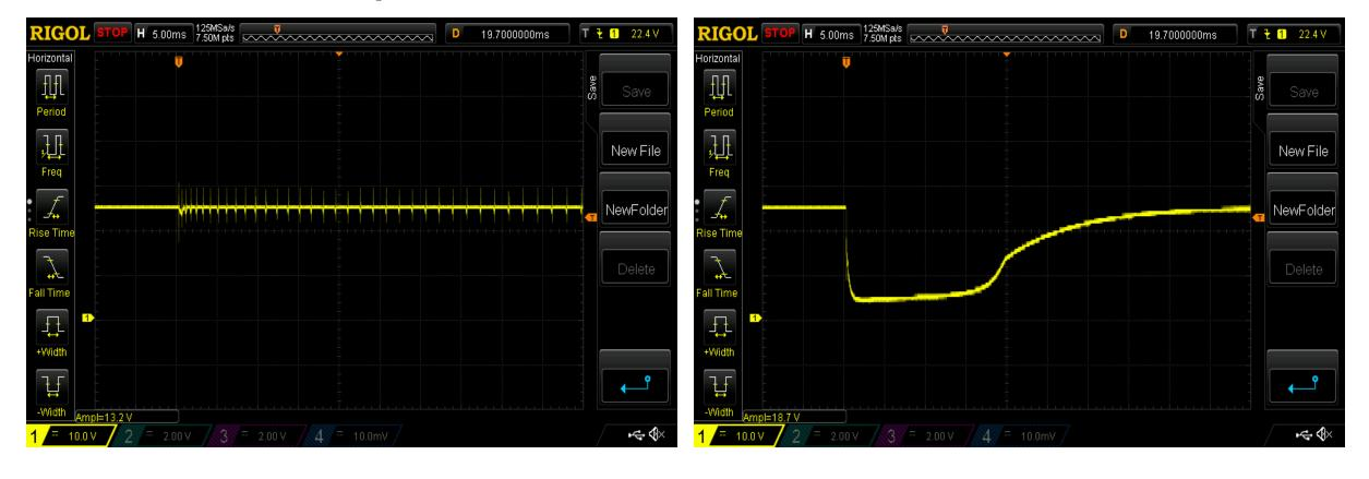
The eFuse (left) responds much quicker then the PTC (right), preventing the input rail from sagging during a fault.
